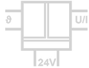
The KTY Temperature Transmitter DT 45600 is used for measure industrial process signals. It converts KTY sensor signals to isolated standard signals.
